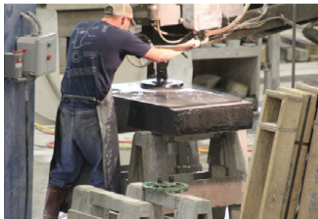
A worker uses a stone grinder that applies water at the work surface to reduce silica dust levels in the air.
