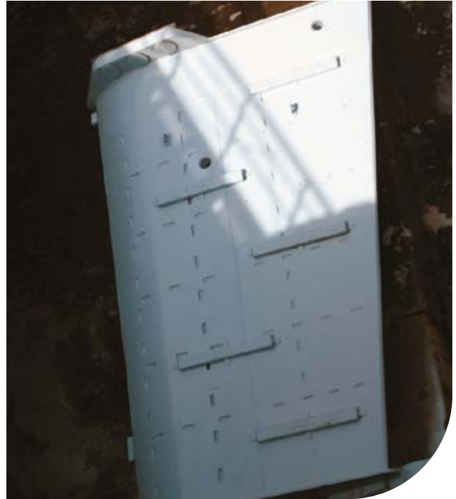
Rudder after application of Chem-glide™ RA 500CG
