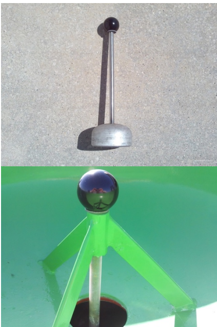
Pot Plunger – This is used to completely seal up the pot. It must be held up until the pump builds enough pressure to maintain the seal. It is located at the top of the pot.
