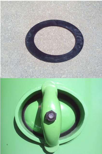
Hand Hold Gasket – The gasket on the service cover of the pot.
